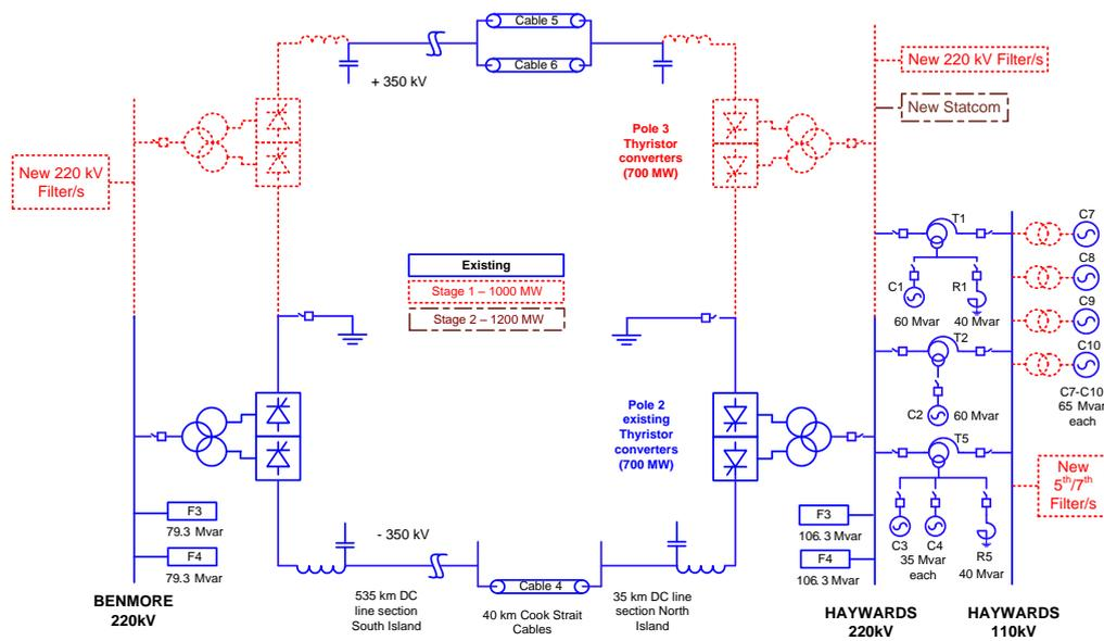
Figure 6-18 shows a simplified diagram for a possible further expansion of the HVDC link to 1,400 MW north capacity following completion of the Pole 3 project. This would involve the installation of:
