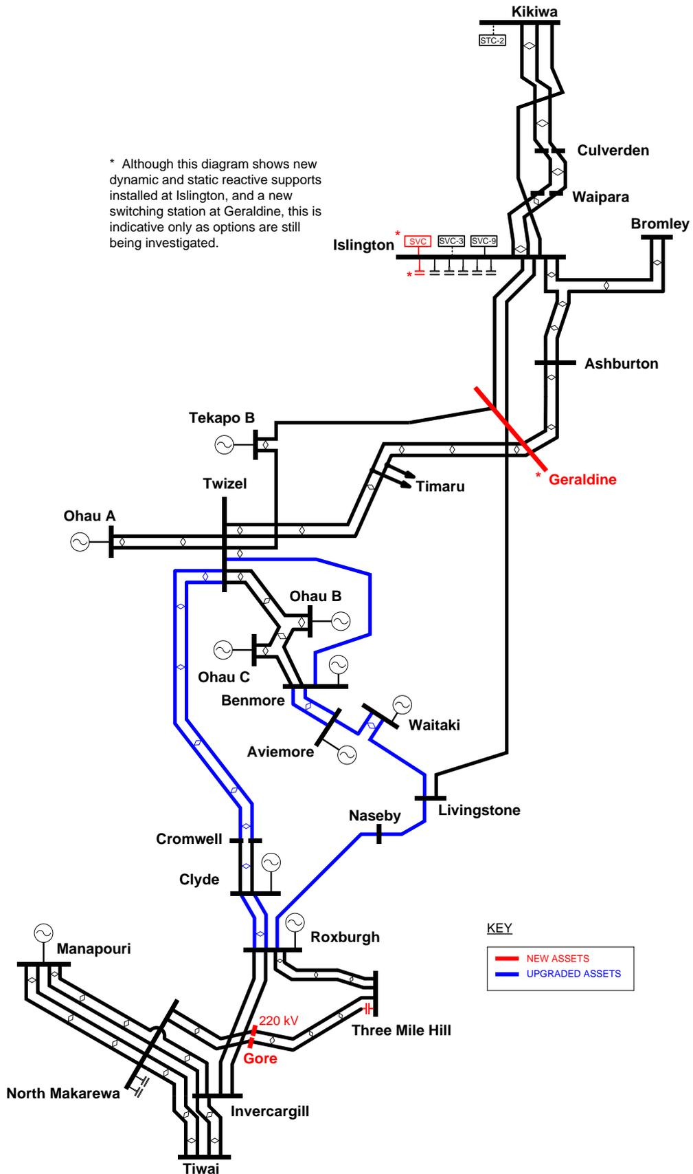
Figure 6-12: Longer term indicative South Island grid backbone schematic
