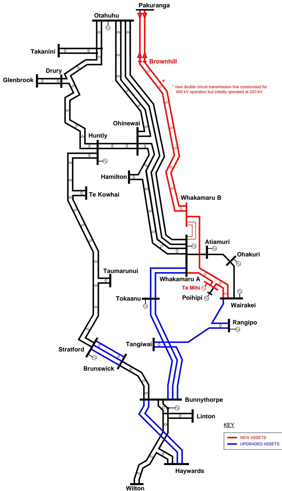
Figure 6-3: Longer term indicative North Island grid backbone schematic
